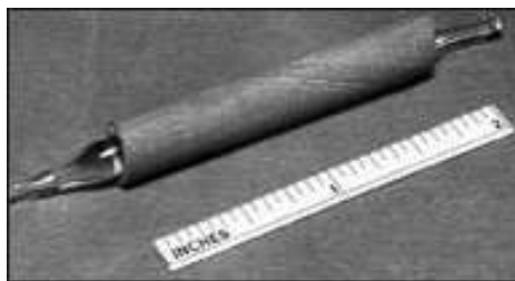
Capsule containing sulphuric acid encased in a rubber tubing for protection
